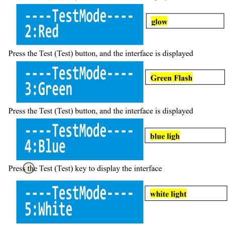
Step 8: After the test is completed, press the loop (OK) key and return to the main interface. (Note: Mode 2, 3, 4 and 5 can be used to test the channel sequence of the lamp.)
