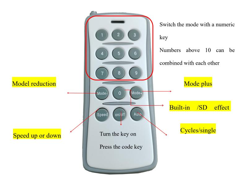
1. The controller and remote have already been calibrated at the factory, with "code alignment labels" attached as shown in the figure below: ID: 1384. A remotely calibrated device can only be used for this specific controller. The remote cannot be used on controllers without the "code alignment label." When using a remote on different labeled controllers, we need to recalibrate,
